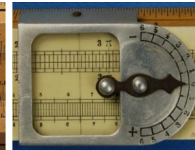
Aluminium, digit registering with 2 domed rivets, rounded window, centre riveted spring
